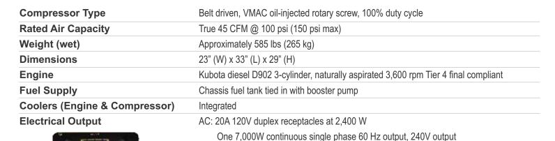
DC: (for battery boost/charging, other DC loads) 12V, 24V, 36V, 48V selectable, 300 A capable
