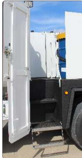
**New center deck access - wider with illuminated stairway and 3-point contact**
